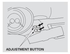
Adjust the brightness of the instrument panel by pressing the + or - button. Press the + button to increase the brightness and the - button to decrease it. You can adjust the brightness with the headlight switch on or off
