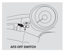
This switch is at the right side of the left vent. Press it to turn the AFS on and off. When AFS is off, the AFS indicator comes on as a reminder when you turn on the headlights.
