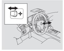
Release the switch when the steering wheel reaches the desired position. Make sure the steering wheel points towards your chest, not toward your face, and that you can see the instrument panel gauges and indicators.
