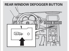
The rear window defogger clears fog, frost, and thin ice from the window. Push the defogger button to turn it on and off. Pushing this button also turns the mirror heaters on and off. The indicator in the button comes on to show the defogger is on. If you do not turn it off, the defogger will shut itself off after 5 to 40 minutes (depending on the ambient temperature). It also shuts off when you turn off the ignition switch. You
