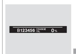
Press the SEL/RESET button on the steering wheel repeatedly to select the engine oil life minder, the message "CHANGE OIL" along with the percentage "0%," and the maintenance item code are displayed on the lower part of the multi-information display when the calculated engine oil life is 0-1 percent.
