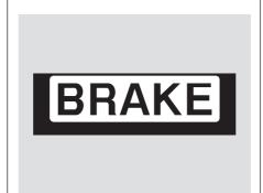
The audible alarm is a constant beeping sound; the visual alarm is an amber colored BRAKE message that flashes in the multi-information display. If these alarms come on, do whatever is necessary to avoid the collision (apply the brakes, change lanes, etc.).
