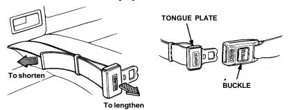
NOTE: When the center lap belt is not in use, store it in the buckle locators as shown.
