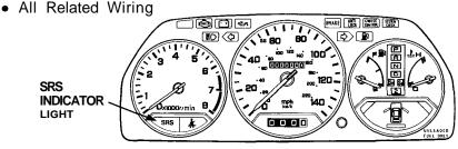
In the event of a malfunction indicated by any of the following, the car should be taken promptly to your nearest Acura dealer to have the system checked. Unless checked and repaired, the SRS will not function reliably:
