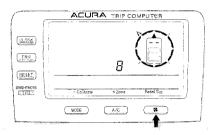
Press the Set ( **%** ) button. "Calibrate" will start blinking, and the direction display will change to "---".
