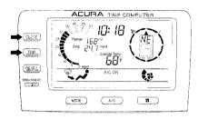
1. Press and hold the CLOCK and TRIP buttons until the display changes (about 1 second).
