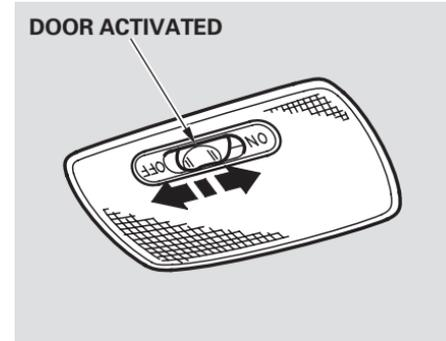
The cargo area light has a three-position switch. In the OFF position, the light does not come on. In the center position, it comes on when you open the tailgate or doors. In the ON position, it stays on continuously.
