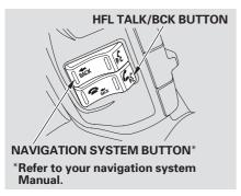
To operate the HFL, use the HFL TALK/BACK button on the left side of the steering wheel.
