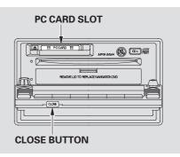
With the ignition in the ACCESSORY (I) or ON (II) position, press the OPEN button, insert a PC card all the way into the card slot, then press the CLOSE button. The PC card will begin to play. You operate the PC card with the same controls used for the radio. The number of the track playing is shown in the display. The system will continuously play a card until you change modes.
