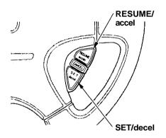
Press and hold the SET/decel button on the steering wheel until the CRUISE CONTROL light on the instrument panel comes on. This shows the system is now activated.
