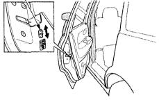
The childproof door locks are designed to prevent children seated in the rear from accidentally opening the rear doors. Each rear door has a lock lever near the edge. With the lever in the LOCK position, the door cannot be opened from the inside regardless of the position of the lock tab. To open the door, pull the lock tab up and use the outside door handle.
