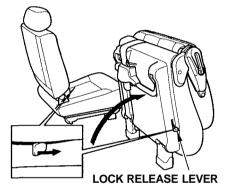
Pull the seat-back angle adjustment lever on the second row seat to tilt the seat-back forward. Pull the lock release lever and pivot the seat up out of the way. Move the second seat back into place by pivoting the seat down. Make sure it locks to the floor. Pull the seat-back angle adjustment lever forward and push the seat-back to the desired position, then release the lever. Make sure the seat is securely locked in place.
