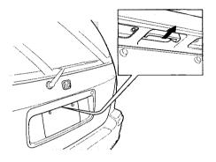
Use your key to lock and unlock the tailgate. (On the U.S. EX model, your remote transmitter will also lock and unlock the tailgate.)
