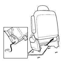
Unhook the front of the seat from the floor by pulling it back slightly, then pivoting it upward.
