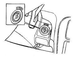
The ignition switch is on the right side of the steering column. It has four positions:
