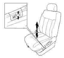
U.S. EX model only The height of your driver's seat is power adjustable. Pull up on the switch to raise the seat. Push it down to lower the seat.
