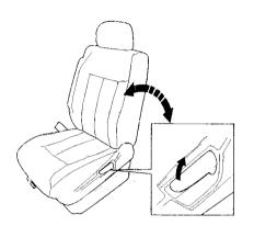
Adjust the seat-back before you start driving. The seat-backs should be in an upright position for you and your passengers to get the most protection from the seat belts.
