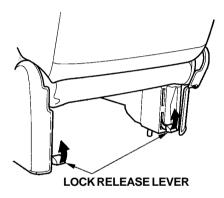
Both seats can be removed to give more cargo capacity.
