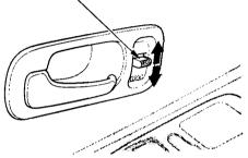
Each front door has a master door lock switch. Either switch locks and unlocks all doors. Push the switch down to lock all doors, and up to unlock them. The lock tab on the tailgate also locks and unlocks when you use the master door lock switch.
