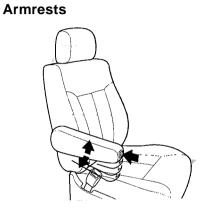
To adjust the front seat armrests, push the button on the front.
