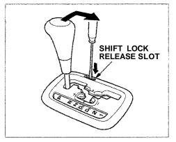
6. Remove the screwdriver from the shift lock release slot, then install a new cover.
