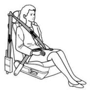
For added protection, the front seat belts are equipped with automatic seat belt tensioners. When activated, the tensioners immediately tighten the belts to help hold the driver and a front passenger in place.
