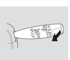
To clean the windshield, pull back on the wiper control lever. The washers spray until you release the lever.
