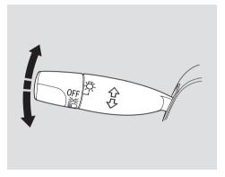
To signal a lane change, push lightly on the turn signal lever in the proper direction and hold it. The lever will return to the center position as soon as you release it.
