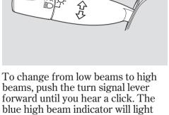
beams, push the turn signal lever forward until you hear a click. The blue high beam indicator will light (see page 59). To return to low beams, pull the turn signal lever back.
