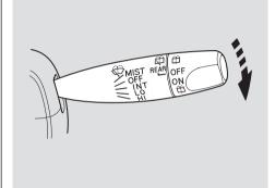
The right lever controls the windshield wipers and washers. The rotary switch at the end of the lever has five positions; MIST: mist OFF: off INT: intermittent LO: low speed HI: high speed
