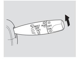
In intermittent, the wipers operate every few seconds. In low speed and high speed, the wipers run continuously.
