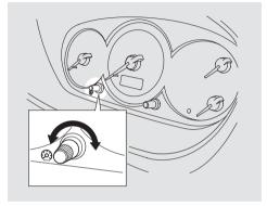
The knob on the instrument panel controls the brightness of the instrument panel lights. Turn the knob to adjust the brightness.
