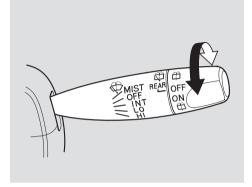
The rotating switch on the right lever controls the rear window wiper and washer.
