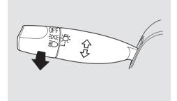
To flash the high beams, pull the turn signal lever back lightly, then release it. The high beams will come on and go off.
