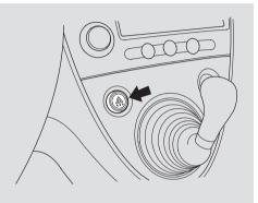
Push the red button to turn on the hazard warning lights (four-way flashers). This causes all four outside turn signals and both indicators in the instrument panel to flash. Use the hazard warning lights if you need to park in a dangerous area near heavy traffic, or if your car is disabled.
