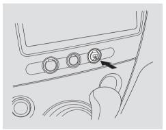
The rear window defogger will clear fog, frost, and thin ice from the window. Push the defogger button to turn it on and off. The light in the button lights to show the defogger is on. If you do not turn it off, the defogger will shut itself off after about 15 minutes. It also shuts off when you turn off the ignition. You have to turn it on again when you restart the car.
