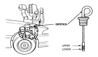
Insert the dipstick and remove it. The fluid level should be between the upper and lower marks.
