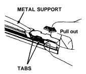
3. Remove the metal retainers from the worn-out blade rubber and put them in a new blade rubber.
