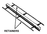
Insert the new blade rubber from the opposite side of the blade tabs and position the tabs in the metal support. The condition of the battery can be determined by checking the test indicator. Service as required according to the label on the battery.
