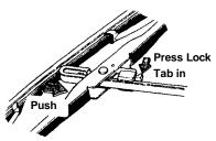
2. Firmly grasp the end of the blade rubber and pull until the tabs are free of the metal support.
