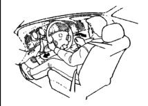
To avoid transmission damage, come to a complete stop before shifting into Park. The shift lever must be in Park before you can remove the key from the ignition switch.
