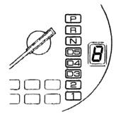
This indicator in the tachometer shows which position the shift lever is in. The illuminated number next to the "D<sub>5</sub>" indicator shows you the gear you have selected in the Sequential SportShift mode.
