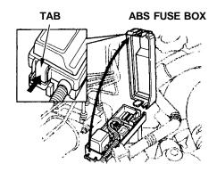
2.5 TL The fuse box for the ABS is located in the engine compartment on the passenger's side. To open it, push the tab as shown.
