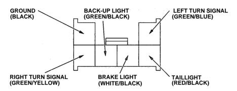
Your car has a trailer lighting connector in the trunk. To use the connector, remove the fastener on the side of the trunk and pull the lining back (see page 232). Refer to the drawing above for the wiring color code and purpose of each connector pin.
