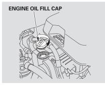
Unscrew and remove the engine oil fill cap on top of the valve cover. Pour in the oil slowly and carefully so you do not spill. Clean up any spills immediately. Spilled oil could damage components in the engine compartment. Reinstall the engine oil fill cap, and tighten it securely. Wait a few minutes, and recheck the oil level on the engine oil dipstick. Do not fill above the upper mark; you could damage the engine.
