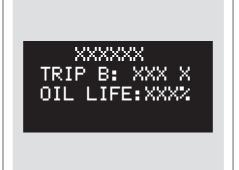
The remaining engine oil life is displayed on the Multi-Information Display as a percentage when you turn the ignition switch to ON (II).
