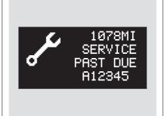
If the indicated maintenance service is not done and the remaining engine oil life gets less than 0 percent, you will see the message, "SERVICE PAST DUE" on the display. Immediately have the service performed, and make sure to reset the display as previously described.
