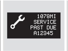
If the indicated maintenance service is not done and the remaining engine oil life gets less than 0%, you will see the message "SERVICE PAST DUE" on the display. Immediately have the service performed, and make sure to reset the display as previously described.
