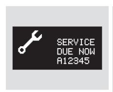
When the remaining oil life is less than 5%, you will see the message "SERVICE DUE NOW" with the same maintenance items you saw when "SERVICE DUE SOON" was displayed. When you see this message, have the indicated maintenance performed as soon as possible.
