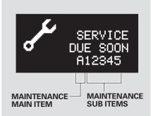
When the remaining engine oil life is 15%, you will see the message "SERVICE DUE SOON" along with all maintenance items that are needed at oil change time. Refer to page 209 for a complete list of the maintenance main items and sub items.
