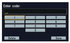
Enter the four-digit navigation system security code, then select **Done**. If you have entered it correctly, the display changes to the **Disclaimer** screen. You have ten chances to enter the correct code. If all ten are incorrect, turn the ignition to OFF, then back to ON (II) to have ten more chances to enter the correct code.
