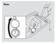
None of the sockets will power an automotive type cigarette lighter element. When more than one socket is being used, the combined power rating of the accessories should be 120 watts or less (10 amps).
