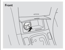
To use the accessory power socket, pull up the cover. The ignition switch must be in the ACCESSORY (I) or ON (II) position.
