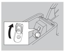
Your audio system will accept auxiliary inputs from a portable cassette player, MP3 player, etc. To use the jack, turn down the volume of the portable unit, and pivot the cover up, then plug in a mini-jack cable between the portable unit and the jack. You will see AUX in the display and the system automatically switches to AUX mode. To adjust the volume, turn the VOL/PWR knob.
