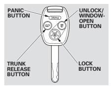
On all models except U.S. DX You can lock and unlock your car with the remote transmitter. When you push the LOCK button, all doors lock. The parking lights, side marker lights, and taillights flash once. When you push the LOCK button a second time within 5 seconds after you have locked the doors, you will hear a beep to verify that the doors are locked and the security system has set.
