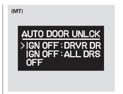
On models with manual transmission Select the condition and door(s) to unlock by moving the pointer with INFO (▼) button and enter your selection by pressing the SEL/RESET button.
