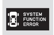
If there is a problem with the TPMS, the tire pressure monitor shows a "SYSTEM FUNCTION ERROR" message and the tire pressure readings are not displayed. If this happens, you will first see a system warning message "CHECK TPMS SYSTEM" on the multi-information display.
