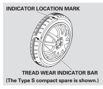
Replace the tire when you can see the tread wear indicator bars. The replacement should be the same size and design tire, mounted on the same wheel. The spare tire is not designed to be mounted on a regular wheel, and the spare wheel is not designed for mounting a regular tire.
