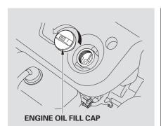
Unscrew and remove the engine oil fill cap on top of the valve cover. Pour in the oil slowly and carefully so you do not spill. Clean up any spills immediately. Spilled oil could damage components in the engine compartment. Install the engine oil fill cap, and tighten it securely. Wait a few minutes, and recheck the oil level (see page 238). Do not fill above the upper mark; you could damage the engine.
