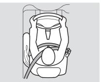
If you ever have a moderate to severe side impact, sensors will detect rapid acceleration and signal the control unit to instantly inflate either the driver's or the passenger's side airbag and activate the seat belt tensioner on that side of the vehicle
