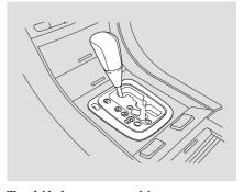
To shift from any position, press firmly on the brake pedal. You cannot shift out of Park when the ignition switch is in the LOCK (0) or ACCESSORY (I) position.
