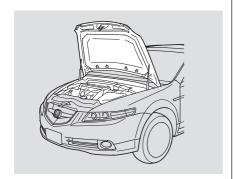
To close the hood, lower it to about a foot (30 cm) above the fender, then press down firmly with your hands. Make sure the hood is securely latched.
