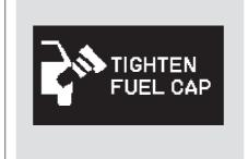
Your vehicle's on board diagnostic system will detect a loose or missing fuel fill cap as an evaporative system leak. The first time a leak is detected a "TIGHTEN FUEL CAP" message appears on the multi-information display. Turn the engine off, and confirm the fuel fill cap is installed. If it is, loosen it, then retighten it until it clicks at least once. The message should go off after several days of normal driving once you tighten or
