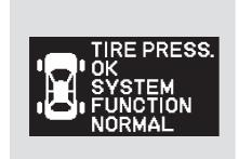
When the tire pressure monitoring system (TPMS) is functioning normally and the tires are properly inflated, you will see the above display on the multi-information display as it cycles through its main menu.
