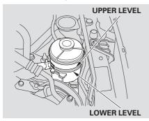
Check the level on the side of the reservoir when the engine is cold. The fluid should be between the UPPER LEVEL and LOWER LEVEL. If not add power steering fluid to the UPPER LEVEL mark.
