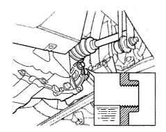
Remove the transmission filler bolt and carefully feel inside the bolt hole with your finger. The fluid level should be up to the edge of the bolt hole. If it is not, add Honda Manual Transmission Fluid (MTF) until it starts to run out of the hole. Reinstall the filler bolt and tighten it securely.
