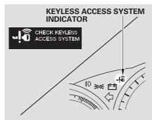
The indicator comes on for several seconds when you turn the ignition switch to the ON (II) position. Have your vehicle checked by your dealer if:
