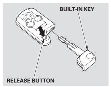
The built-in key can be inserted into the remote.
