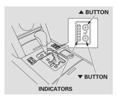
Both front seats are equipped with seat heaters and an air ventilation system. The passenger seat only has heaters in the seat bottom because of the side airbag system. The ignition switch must be in the ON (II) position to use the heaters and the air ventilation system.
