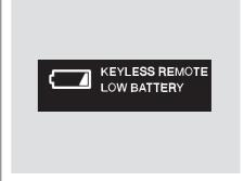
The batteries in the remote normally lasts about 2 years. To ensure maximum battery life, do not store the remote close to electrical devices such as computers or TVs. When the multi-information display shows "KEYLESS REMOTE LOW BATTERY," replace the batteries as soon as possible (see page 167).
