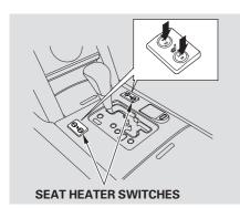
Both front seats are equipped with seat heaters. The passenger seat only has heaters in the seat bottom because of the side airbag system. The ignition switch must be in the ON (II) position to use the heaters. Push the top of the switch, HI, to rapidly heat up the seat. After the seat reaches a comfortable temperature, select LO by pushing the bottom of the switch. This will keep the seat warm.
