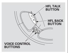
To operate the HFL, use the HFL Talk and Back buttons on the left side of the steering wheel. Below the HFL buttons is another set of voice control buttons for the navigation, climate control, and audio systems.
