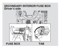
To open the secondary fuse box lid, push the tab in the direction shown in the illustration.
