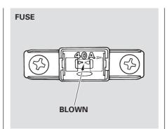
3. Check each of the large fuses in the under-hood fuse box by looking through the top at the wire inside. Removing these fuses requires a Phillips-head screwdriver.
