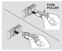
4. Check the smaller fuses in the under-hood fuse box and all the fuses in the interior fuse boxes by pulling out each fuse with the fuse puller. The fuse puller is inside the primary under-hood fuse box.
