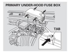
The primary under-hood fuse box is in the engine compartment on the driver's side. To open it, push the tabs as shown.
