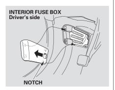
The fuses are located in five fuse boxes. The interior fuse boxes are located under the dashboard on the driver's and passenger's side.
