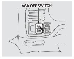
This switch is under the left vent. Press it to turn the Vehicle Stability Assist system on and off.
