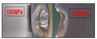
Tensile Test Results of Welded 1,500 MPa Steel
