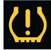
Low Tire Pressure/TPMS Indicator
