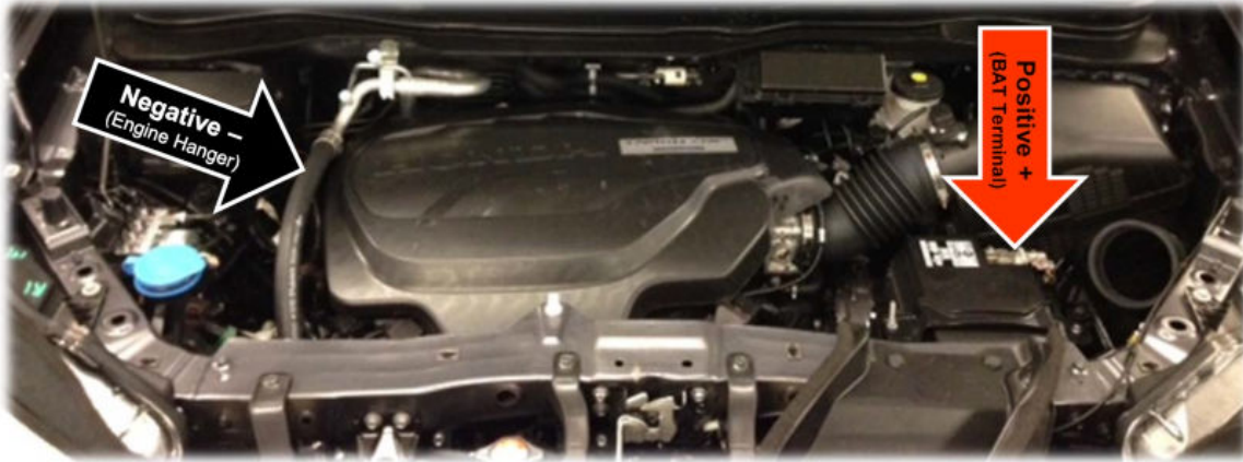
12-Volt Battery Under Hood Jump Starting/Charging/Testing Locations
