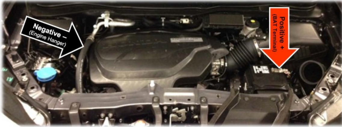
12-Volt Battery Under Hood Jump Starting/Charging/Testing Locations
