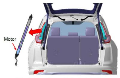
Spindle-Type Power Tailgate Actuator
