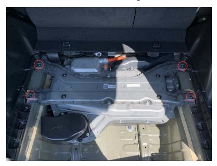
NOTE: When doing repairs in this area (rear upper frame, upper stiffener), do not primer or paint the areas indicated below. In addition, make sure those areas are free of corrosion.
