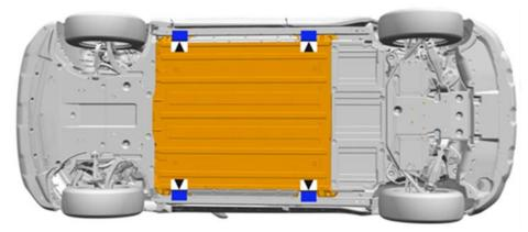
Make sure to remove the Rocker Panel Molding Jacking Opening Front Cover before positioning the lift onto the vehicle.
