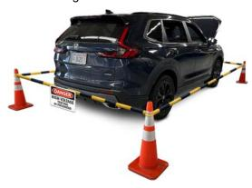
When removing the high-voltage battery, designate an area of the shop where it can be safely stored during repairs. A buffer zone should also be created, and cones placed for safety.
