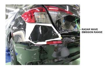
To assist technicians in determining where the radar wave emission area is, a printable template is provided in the body repair manual. This template can be taped onto the bumper and will help determine if the bumper can be repaired or will require replacement.
