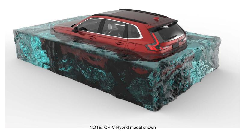
Aside from severe damage to the vehicle, there is no risk of an electric shock from touching the vehicle's body or framework - in or out of the water. If the high-voltage battery was submerged, you may hear noises from the battery as the cells are being discharged from shorting.
