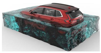
5. Continue filling the pool to a minimum depth of **2.41 feet (734 mm)** until the high voltage battery is completely submerged.
