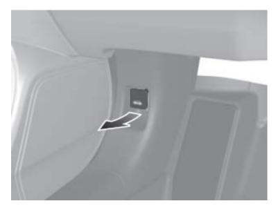
2. Locate the hood latch lever, pull the lever, and lift the hood.
