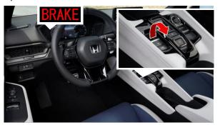
2. Press the brake pedal and press the **P** button.
