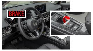
2. Press the brake pedal and shift to P.
