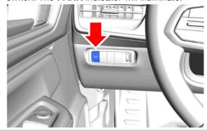
2. Press the brake pedal, then press the button at the end of the shift lever to shift to P (Park).
