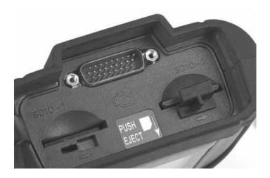
2. Push the SD card inward and release. The SD card releases and partially ejects.
