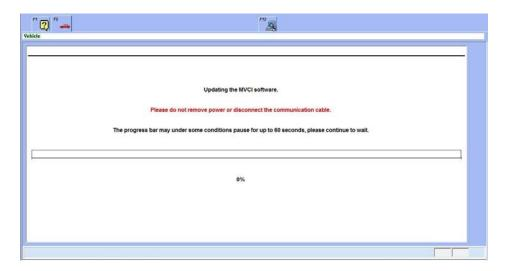
4. The MVCI automatically reboots. Follow the directions on the HDS screen. Do not disconnect the external power source or disconnect the MVCI from the PC.
