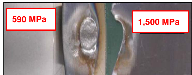
Tensile Test Results of MAG-Welded 1,500 MPa Steel
