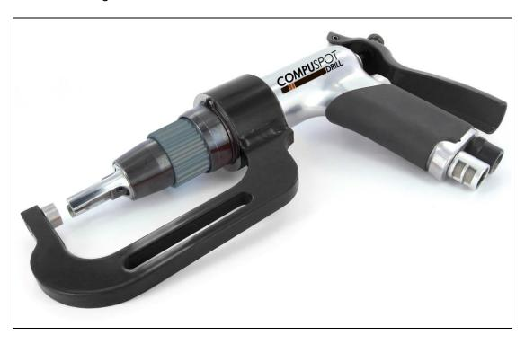
A special transmission delivers high torque at reduced RPM in order to prevent overheating the carbide bits. This is done without the need to reduce the incoming air pressure (which would result in the loss of torque).
