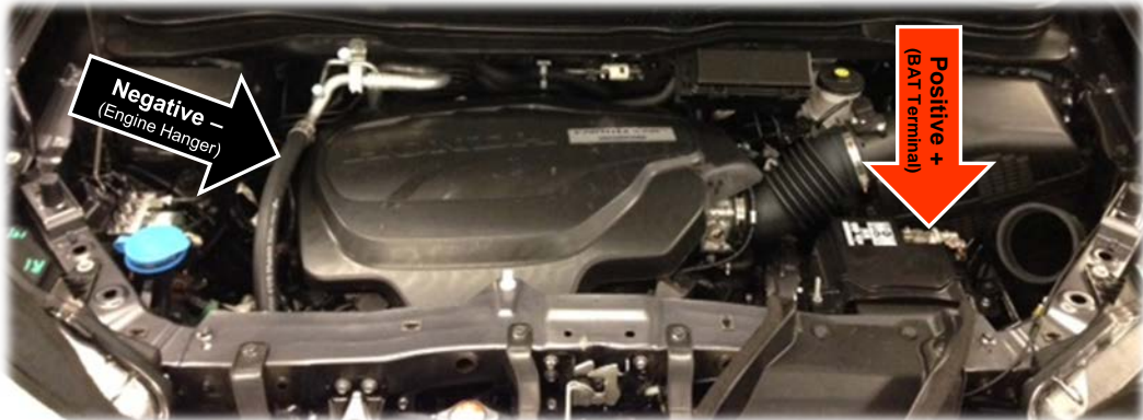
12-Volt Battery Under Hood Jump Starting/Charging/Testing Locations
