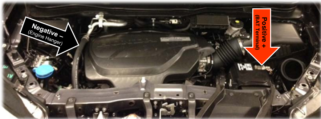
12-Volt Battery Under Hood Jump Starting/Charging/Testing Locations
