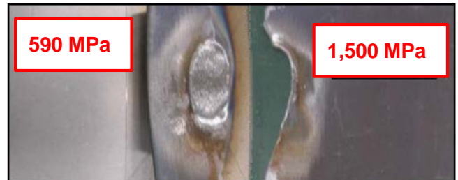
Tensile Test Results of MAG-Welded 1,500 MPa Steel
