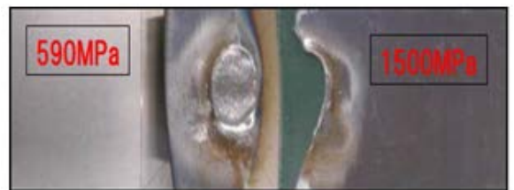
Tensile Test Results of Welded 1500 MPa Steel
