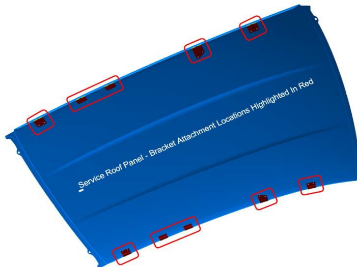
Service Replacement Roof Panel (Underside View)
